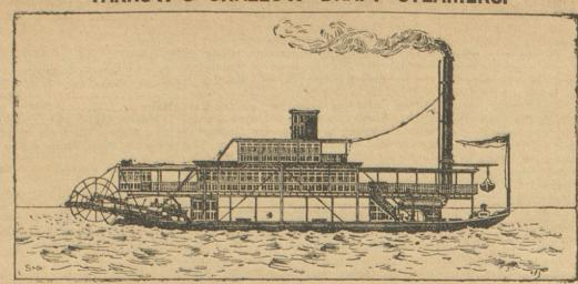
STERNWHEEL STEAMERS have been found by experience to be the best type of vessel for shallow river navigation, and of these Messrs. Yarrow have constructed a large number of successful examples for all parts of the world.
