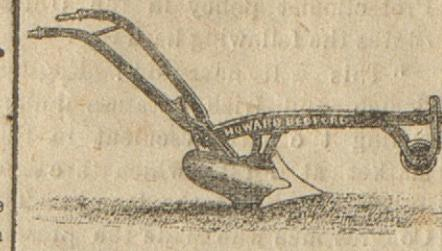
A small, light hill side, turnwrest, or one way Plough, made both with wood and iron beams and handles. The breast and share are attached to pivots, and on coming to the end of the land, the ploughman reverses the breast for the return furrow, the share moving into position at the same time acts also as a coulter.
