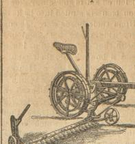
With two Knives, Seat and Tool Box, containing all requisites for use in the field, weight 10½ cwt ......
